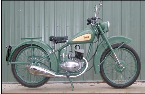
**Stock 1949 BSA 125 Bantam, note the pillion rack, rigid rear frame, absence of rear seat and rear foot-pegs.**
