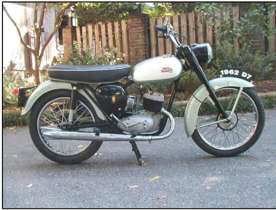
**Mid 60's Bantam D7, note Swinging Arm suspension, Rear Foot-pegs and Dual Seat.**
