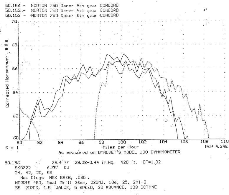
28.18-0.73 in.Hg. 420 ft. CF=1.05 91.1 F 50.152 5.75' AU 950722 24, 42, 20, 58 New Plugs MGK 89EG, .035 . MORRIS 480, Amai Mk II 36mm, 230MJ, 106, 25, 2A1-3 55 PIPES, 1.5 VALUE, 5 SPEED, 30 HOWANCE, 109 OCTANE 29.29-0.73 in.Hg. 420 ft. CF=1.04 50.153 90.5 °F 6.75' 960722 RW 24, 42, 20, 59 New Plugs NGK B9EG, .035. NORRIS 480, Amal Mk II 36mm, 230MJ, 106, 25, 2A1-3 55 PIPES, 1.5 VALUE, 5 SPEED, 30 ADVANCE, 103 OCTANE
