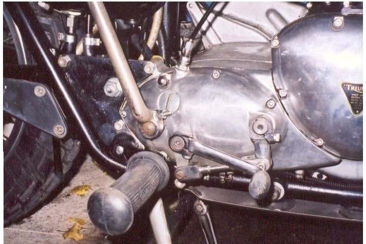
*Figure 6 – Footpegs back 3" using shift linkage*
