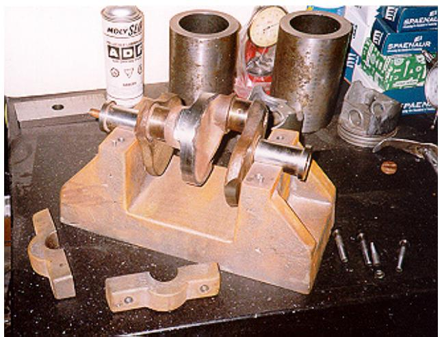
Figure 2 – Crank and fixture
