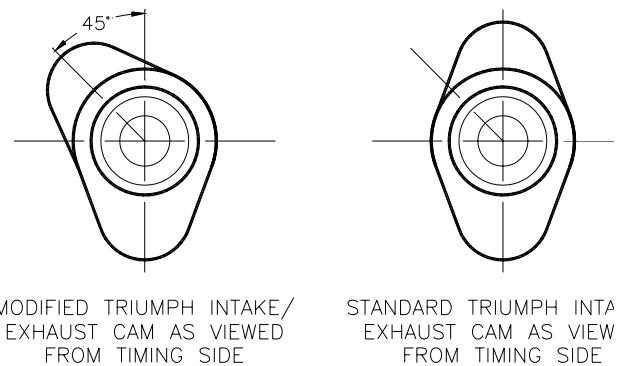
*Figure 4 – Camshaft lobe offset, timing side is standard, drive side is 45 degrees behind*
