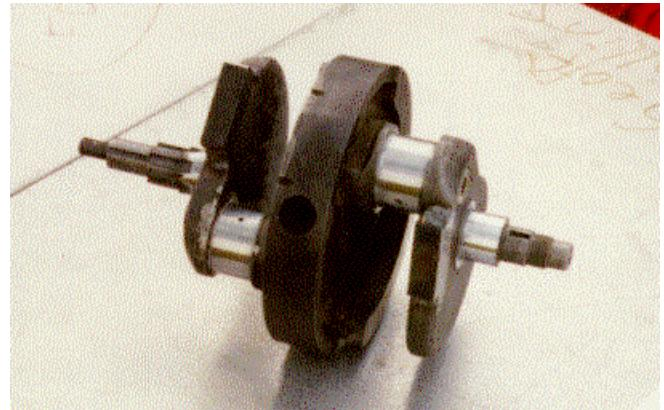
*Figure 3 – The first crankshaft – original flywheel mounting holes are not used..*
